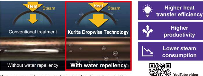
During steam condensation, this technology transforms the water film acting as thermal barrier into droplets to increase heat transfer efficiency.
